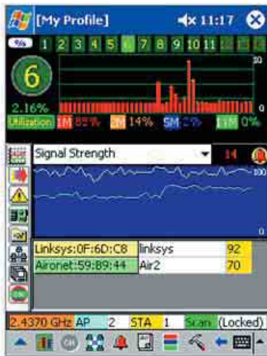
Figure 3. Wireless "sniffing" Palm style with Air Magnet and a HP IPAQ Pocket PC.
