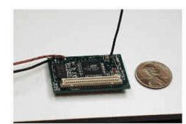
UCB mote: an 8-bit sensor node with non-IP based networking
